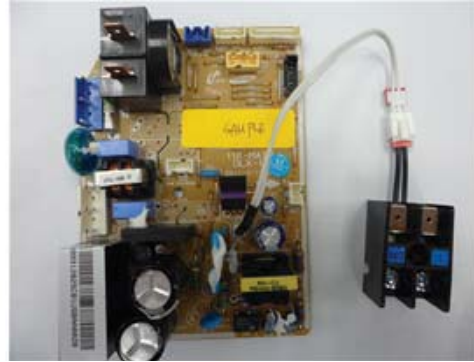
Connection of terminal block and Main PBA
