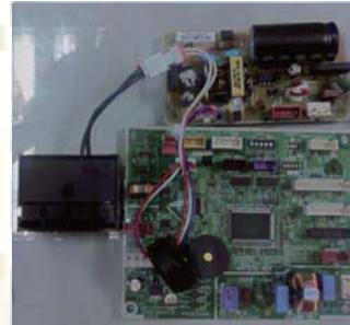
Connection of terminal block and Main PBA
