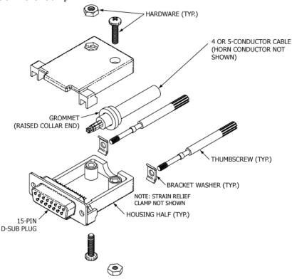
Figure 24 D-Sub Plug Assembly
