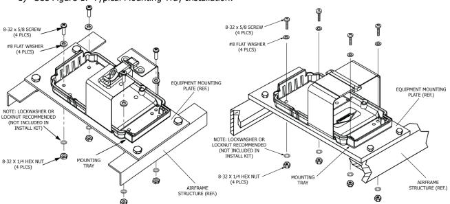
Figure 17 Typical Mounting Tray Installation
