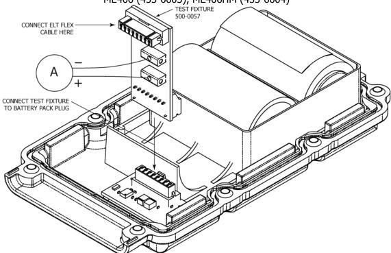
**Figure 10 Current Draw Test Setup**
