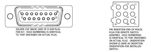
**Figure 21 Metal Airframe Wiring Diagrams**
