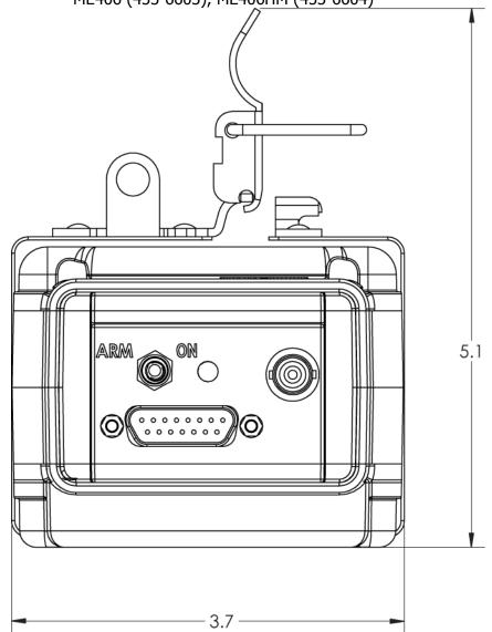
**Figure 16 ME406 Metal Strap Minimum Clearance Dimensions**
