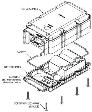
**Figure 27 Battery Pack Installation**
