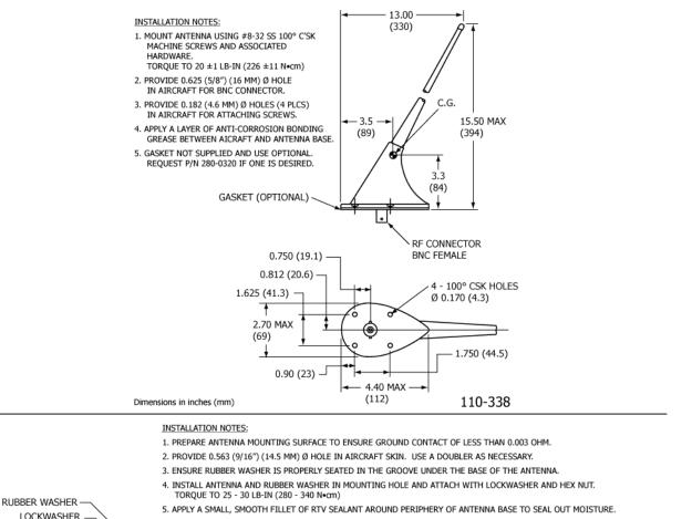
Figure 18 Rod Antenna 110-338 and Whip Antenna 110-773 Outlines and Dimensions
