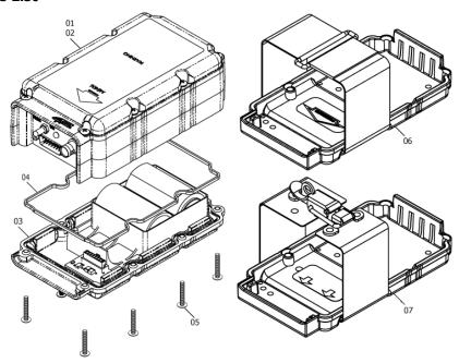
Figure 29 ME406 Series ELT Main Assembly and Installation
