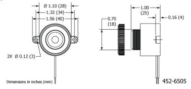
**Figure 20 Buzzer Outline and Dimensions**
