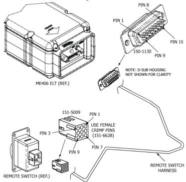
**Figure 23 Remote Switch Harness Arrangement**
