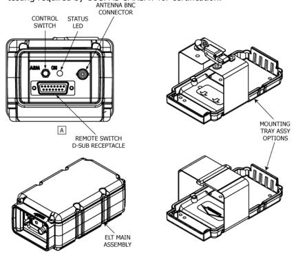
Figure 2 ME406 Series ELT and Mounting Tray Assembly
