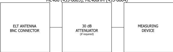
**Figure 9 Performance Testing Equipment Setup**
