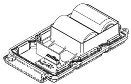
**Figure 5 Battery Pack Assembly**
