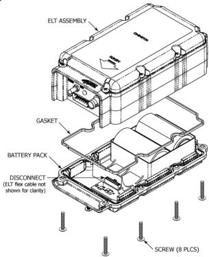
**Figure 14 Battery Pack Removal**
