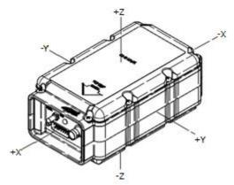
**Figure 28 ELT Orthogonal Axes**
