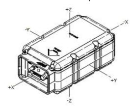
Figure 1 ELT Orthogonal Axes
