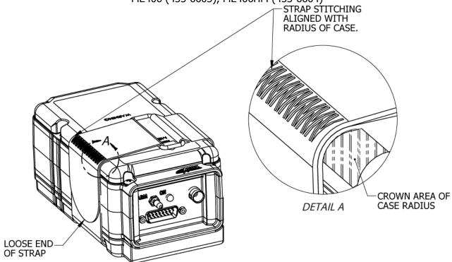
Figure 26 Velcro Strap Installation & Inspection
