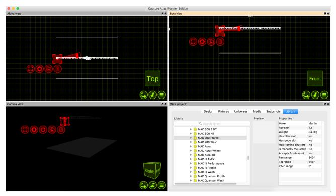
In this example, we add a single Mac 700 profile. We then clone it we end up with one Mac 700 per meter of the truss
