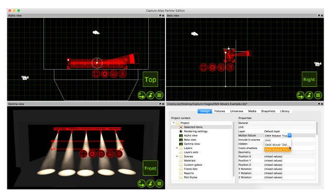
Now, select the DMX Rotator and in the "Motion Fixture" property, assign the Rotator to the DMX Mover. This "Chains" the two motion controllers together so that when we select both, the truss can be moved up and down and rotated at the same time.
