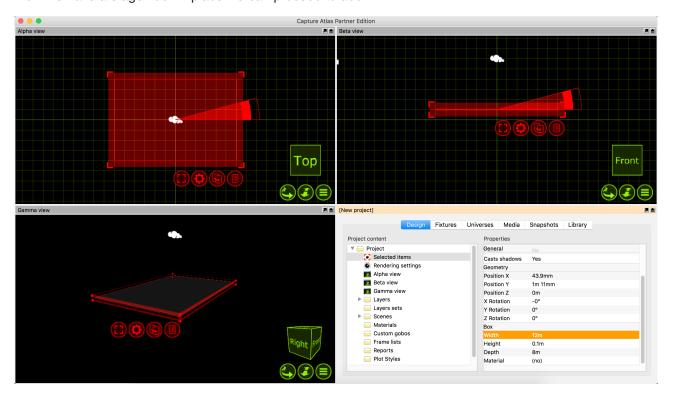
some more objects. We will add some truss in above the stage. Adding a piece of truss is done in the same way the box was added. Locate the desired piece in the library and drag it into either the Alpha are Beta view. For the sake of example, we will use a piece of truss from the **Generic** folder. Double click the **Truss** folder, double click again on the **Generic** folder, and again on **Box**. Choose the **Generic Rectangular Section** and drag it into one of the views.
