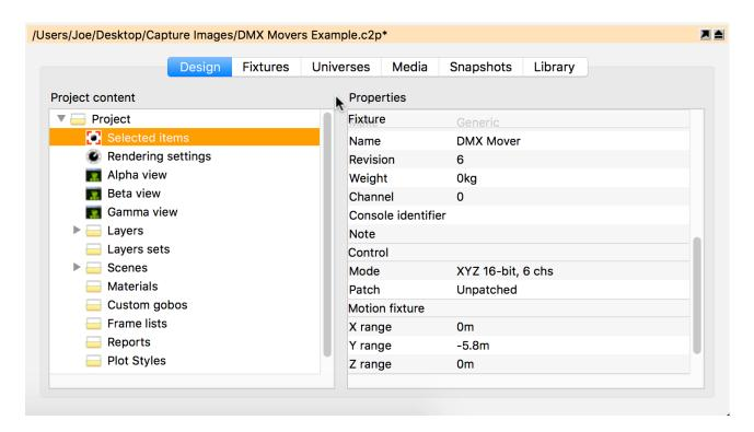
Select the Truss and the Fixtures you wish to move and select the DMX Mover from the "Motion Fixture" property in the Project Window.
