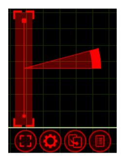
The DMX Mover, pictured to the left, has two blobs at each end of the range. The thicker blob indicates the default starting point of the object the Mover is attached to. The thinner blob indicates the lowest point to Mover operates to.
