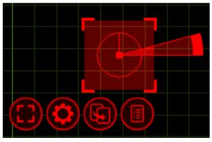
The DMX Rotator, pictured to the left, is shown here as it is seen in the "Orthographic Front" simulator view. The thick blob in the middle of the circle indicates the central rotation point that the object will rotate around. The line protruding from the centre of the circle from the blob is the default starting point. The circle itself indicates the range in which the Rotator can operate. In this case, it is a full circle as the Rotator has a range of 360 degrees.
