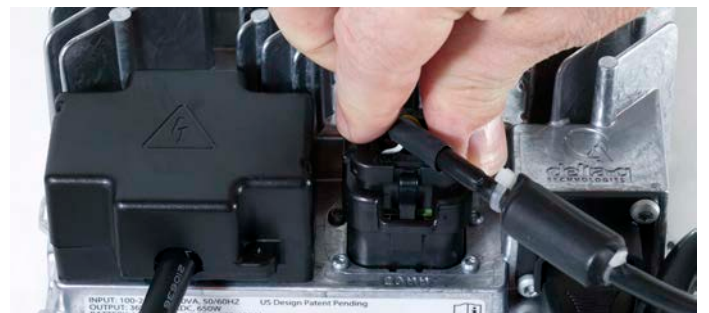
Figure 23. Apply pressure until you hear an audible “click” as the plug locks into position.
