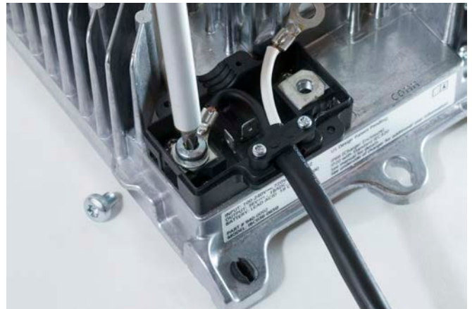
Figure 19. Fix the DC cable in place using the Delta-Q cable clamp, fastened with Torx T10 screws to a recommended torque of 0.6Nm +/-6%. Proceed by attaching the positive and negative leads to the positive and negative terminals, respectively, using the Torx T30 screwdriver and Torx T30 / M6 screws, with a recommended torque of 4.5Nm +/-5%.
