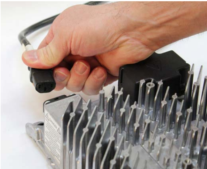
Figure 30. Disconnect AC input from the charger.
