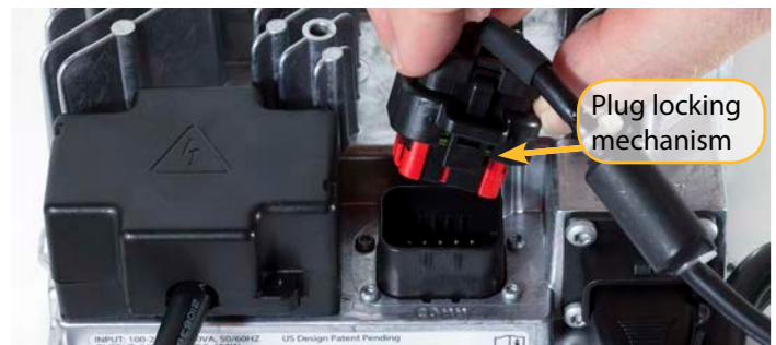
Figure 22. Insert the TE Connectivity AmpSeal Plug into the Comm fixture with the locking mechanism facing toward the outer edge of the charger.
