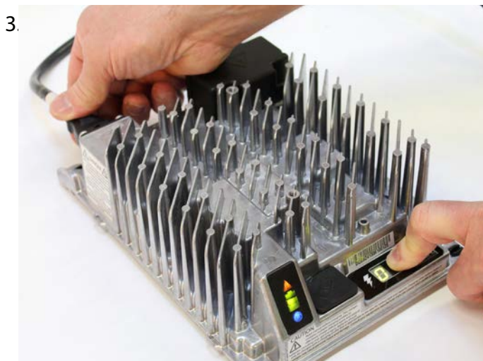
Figure 31. Reconnect AC input while holding the Select Charge Profile Button.
