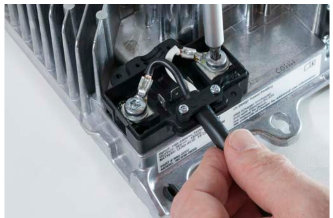
Figure 19. Fix the DC cable in place using the Delta-Q cable clamp, fastened with Torx T10 screws to a recommended torque of 0.6Nm +/-6%. Proceed by attaching the positive and negative leads to the positive and negative terminals, respectively, using the Torx T30 screwdriver and Torx T30 / M6 screws, with a recommended torque of 4.5Nm +/-5%.
