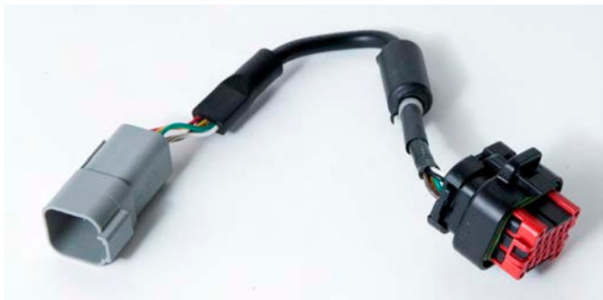
Figure 21. TE Connectivity AmpSeal Plug assembly (Part no. 776273) for onboard communication capabilities, including CAN bus and Modbus.
