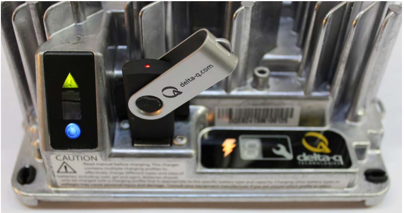
Figure 33. Insert the USB flash drive to begin the charge data download process. This step can be completed using the same USB flash drive programmed to update the charger's software. The process is completed when the USB indicator is solid green, and no longer flashing.
