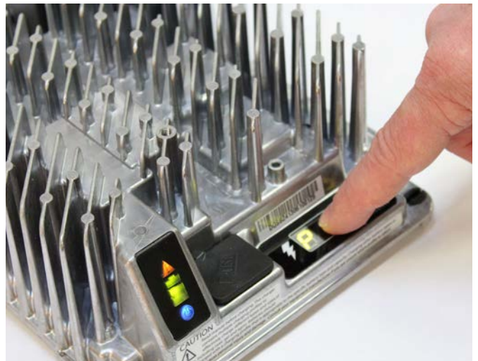
Figure 29. Press the Select Charge Profile Button to advance through the charge profiles. When the desired charge profile appears, hold the button for 10 seconds to confirm your selection.
