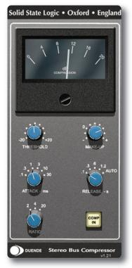
Uses may include inserting the bus compressor over a stereo mix which has the effect of 'gluing' the mix together whilst still maintaining a big sound. The dynamics of drum overheads or whole drum kits can be controlled very effectively with the bus compressor. As it is available as either a stereo or mono plug-in the bus compressor can be used for practically any application that requires superior compression.
