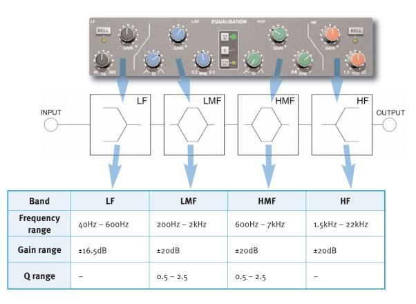
Press the **E** to switch the EQ emulation from G Series to E Series consoles. The diagrams to the right display the difference between them:
