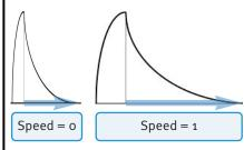
**Speed** controls the length of time the added attack takes to fall back down to the normal signal level once it has reached the top of the attack phase. Turn the knob clockwise for a slower speed, and longer transient.
