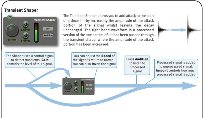
Switch the Shaper on by clicking on the 'power' button in its top left-hand corner. The central meter gives visual feedback on how much attack is being added using the **Gain** and **Amount** controls. If this rises to the top red section then reduce the effect.
