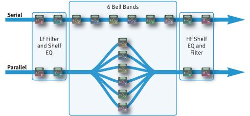
The parallel EQ is modelled on the old 'Parallel Passive' EQ units, and the different style of band interaction means that the EQ performs quite differently. See the EQ History section on Page 41 for more information.
