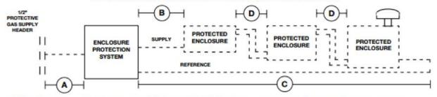
\*NOTE: TUBE AND PIPE SIZES ARE TRADE SIZES AND ARE NOT EQUAL IN INSIDE DIAMETERS. DO NOT SUBSTITUTE TUBE FOR PIPE WITH SAME TRADE SIZE.
