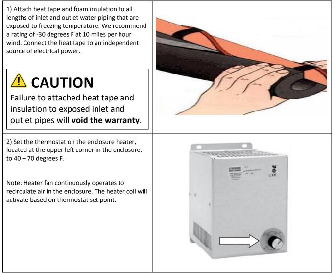
Note: Power must be applied to the water heater for the freeze protection system to operate. If power is not applied ensure the system is completely drained. Neglecting to do so will damage the heater and void the warranty.
