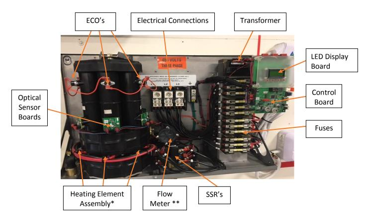
\* HEATING ELEMENT ASSEMBLY CONSISTS OF ONE HEATER CORE AND WIRE ELEMENT(S)
