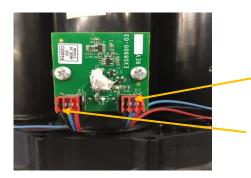
Lead placement: TEST BLUE AND BLACK SEPERATELY. PUT 1 LEAD ON BLUE WIRE ON P5 PLUG THEN OTHER LEAD GOES TO EACH BLUE WIRE ALONG OPTICAL SENSORS. REPEAT WITH BLACK WIRE.
