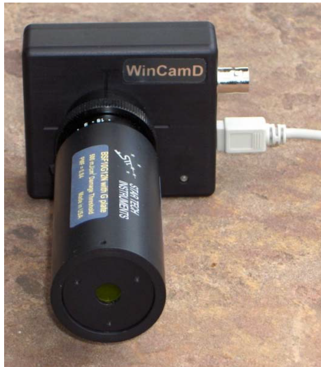
Fig. 5.6: The WinCamD has optional screw-on UV Converters.
