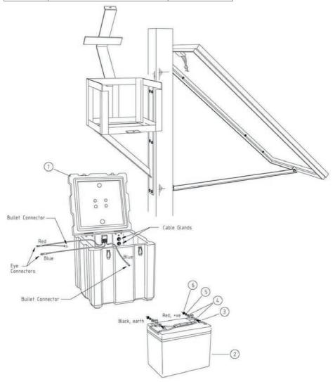
Figure 3. Battery and Battery Box
