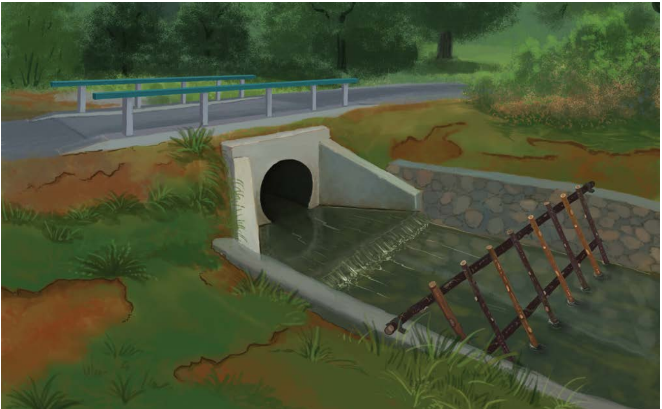
Picture: Trash rack for culverts to prevent clogging
