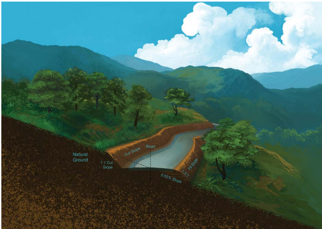
A. Balanced cut and fill
