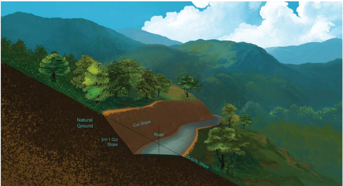
Picture: A typical example of balanced cut and fill for road construction
