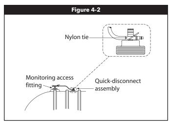
**4.5.3.** The quick-disconnect assembly must not be connected to the service fitting when pressure testing the primary tank. Keep the nylon tie in place.
