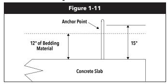
**1.3.6.6.9.** When using our straps and turnbuckles, anchor points must extend at least 3 inches [8 cm] above the bedding. With a 12-inch [30-cm] bedding, the anchor point is 15 inches [38 cm] above the slab.
