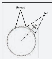
End view of a tank in the rotated position
