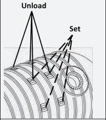
Always hoist a tank with 4 lifting lugs if there are 6 total lifting lugs
