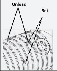
Always hoist a tank with 2 lifting lugs if there are 3 total lifting lugs
