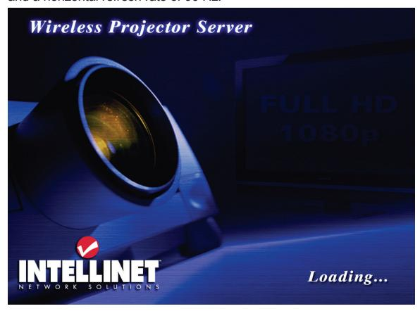
If the above image displays for more than two minutes, turn the Wireless Projector Server off and then on again. If this initial image still remains longer than a couple of minutes, refer to Section 6 Troubleshooting for possible solutions.
