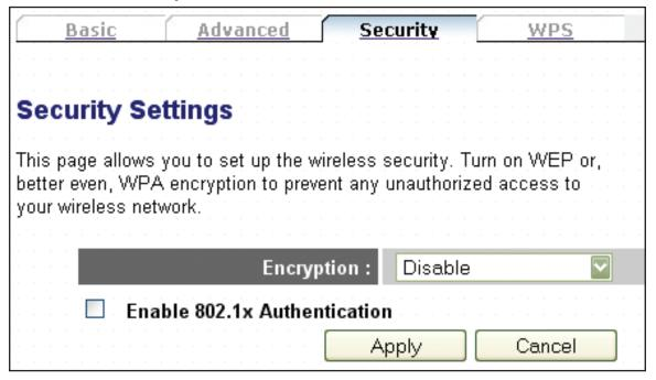
**Encryption:** Select one of four options from the drop-down menu. **NOTE:** Each of these options is explained briefly below, with separate subsections that follow with detailed explanations of the features.
