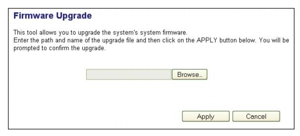
Click "Browse..." to select a firmware file from your computer, then click "Apply" to start the upgrade. The procedure may require some time, so be patient and don't switch your computer or the projector server off during the process. Nor should you remove the network connection during a firmware upgrade: If the upgrade fails, the projector server may not be able to function properly.
