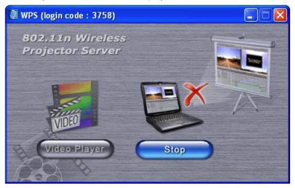
**Stop:** Click to stop the presentation. Your computer's display content will not be transmitted to the projector server's display, but your computer will remain connected (logged in) to the projector server.
