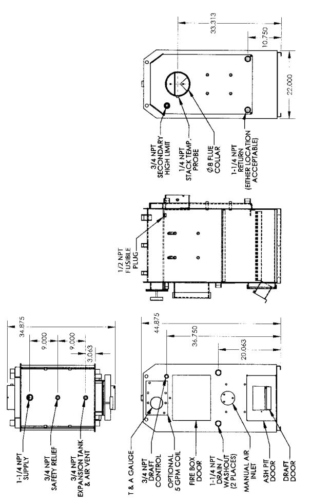
FIG. 3 PIPING CONNECTIONS AND CONTROL LOCATIONS
