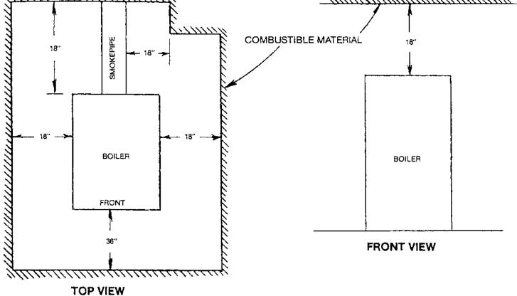
FIG. 2 CLEARANCES TO COMBUSTIBLE MATERIAL
