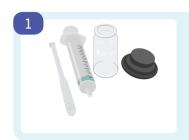
Rinse all equipment thoroughly with the water that is being tested.
