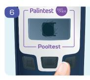
Press the "read sample" key The screen will show that "reading" is in progress.
