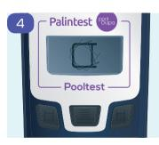
The screen will show that the instrument is measuring the blank.
