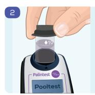
Place a test tube containing pool or spa water (without test tablets) in the cell holder.
