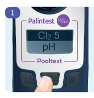
Select a test by pressing the Menu key. Scroll through the list until the desired test is highlighted.
