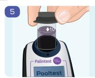
Prepare a 10mL sample by adding reagents according to the Test Instructions. Place this sample tube in the cell holder.
