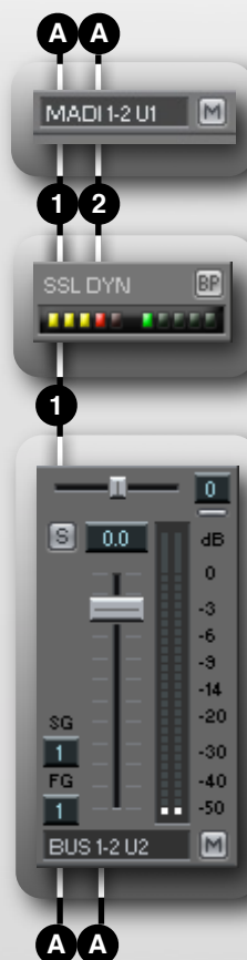
stereo in - mono to stereo out connection diagram
