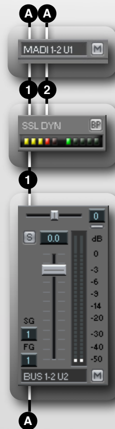
stereo in - mono out mixer strip connection diagram
