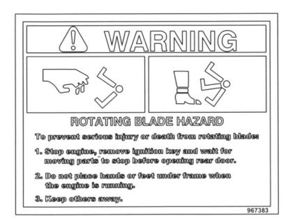
REMEMBER - If Safety Signs have been damaged, removed, become illegible or parts replaced without safety signs, new safety signs must be applied. New safety signs are available from your authorized dealer.
