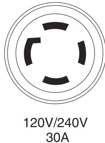
Figure 10 - 120/240 VAC, 30 Amp Receptacle
