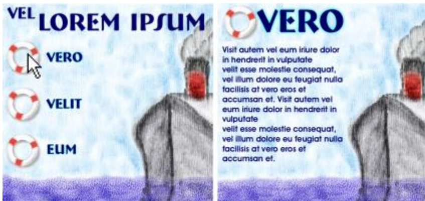
When a hotspot is clicked (left), the browser jumps to the page referenced by that link (right).
