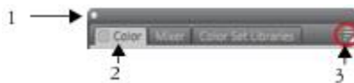
A typical palette features a header bar (1), panel tabs (2), and a Panel options button (3).
