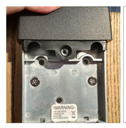
Install the end cap onto the chassis by pressing it over the screw post as shown.
