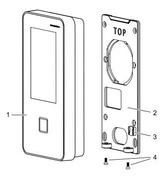
The product consists of the terminal housing (1) and the mounting plate (2).
