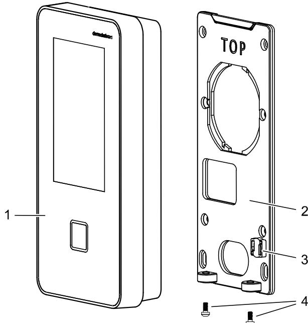
The product consists of the terminal housing (1) and the mounting plate (2).
