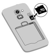
**Tip:** Take care not to scratch or bend the contacts on the memory card or the SIM card when inserting them into the card holders.
