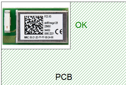
Figure 31: Placing at the edge
