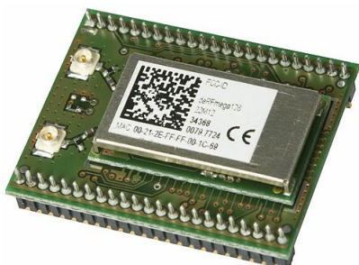
Figure 43: deRFmega128-22T13 with radio module deRFmega128-22M12
