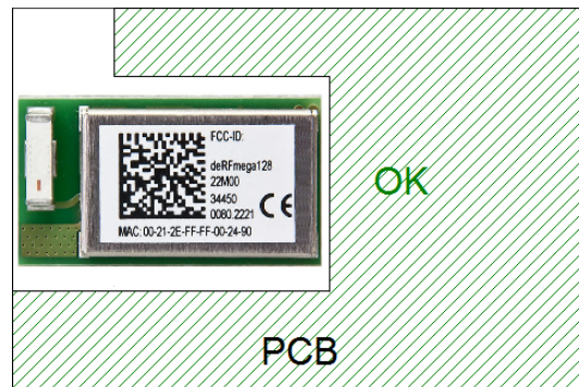
Figure 32: Placing at the center edge
