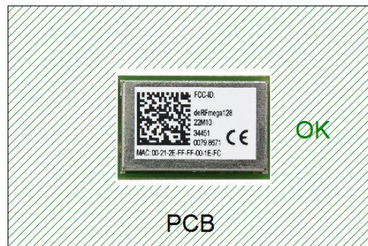
Figure 34: Placing in the center with RF pad
