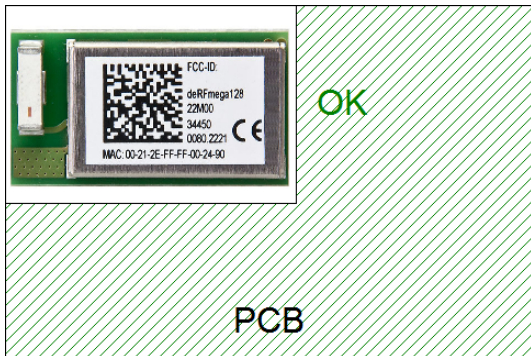
Figure 38: Placing at the edge
