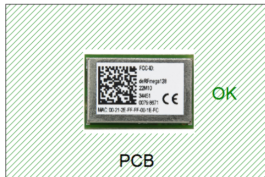
Figure 41: Placing in the center with RF pad
