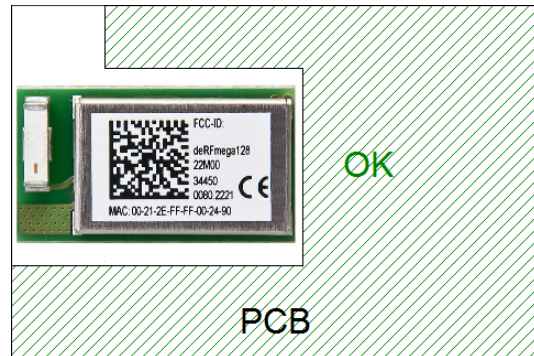
Figure 39: Placing at the center edge
