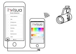
By going to my.invisua.com, one of the pre-stored light scenes can be activated. With the color-picker the fixture(s) can be set to any white or RGB color instantly. (Make sure you are connected to the same network as the Invisua Lightport)
