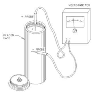
Figure 22. Beacon Off-Current Test Set-Up
