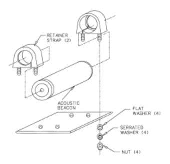
Figure 13. Method of Installing the N30A21A Mounting Kit
