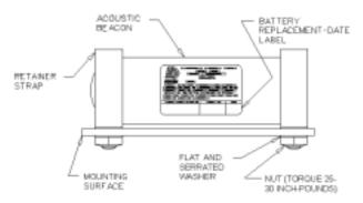
Figure 8. Securing Beacon in N30A21A Mounting Kit
