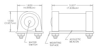
Figure 12. N30A21A Mounting Kit and Beacon Overall Dimensions
