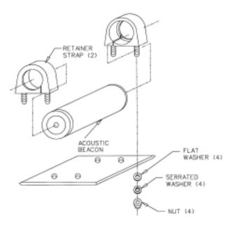
Figure 7. Method of Installing the N30A21A Mounting Kit
