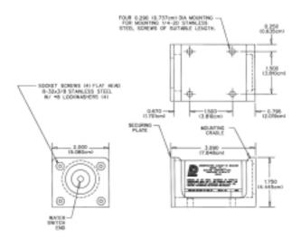
Figure 9. N30A29 Mounting Kit Installation Details
