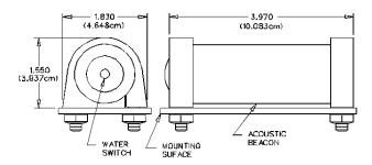
Figure 6. N30A21A Mounting Kit and Beacon Overall Dimensions
