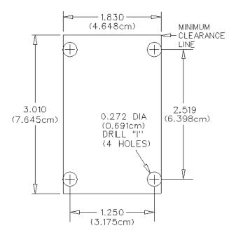
NOTE: ADDITIONAL CLEARANCE IS DESIRABLE AT SWITCH END OF BEACON
