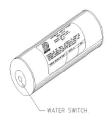
Figure 2. Water Switch Location on Beacon
