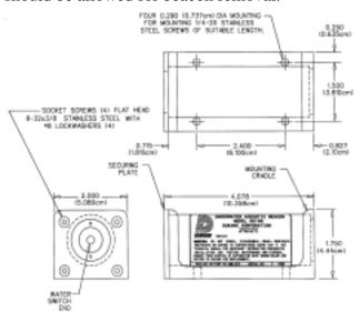
Figure 3. N30A26 Series Mounting Kit Installation Details
