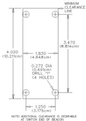
Figure 5. Mounting Hole Template for N30A21A Mounting Kit
