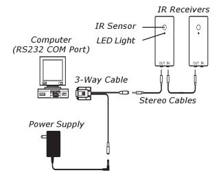
When more than one IR Receiver is required for coverage, plug one end of the 12 meter Stereo Cable into the **OUT**put jack on the second unit and the other into the **IN**put jack on the first unit, the third into the second, and so on down the chain. The last IR Receiver in series does not have to be terminated. One Power Supply will serve up to four units in the chain. Please contact GTCO CalComp if you require a special configuration. Contact information is in the *Appendix*.
