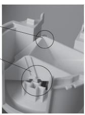
• Insert the rainfall sensor into its holder. It will hold the count rocker firmly automatically.
