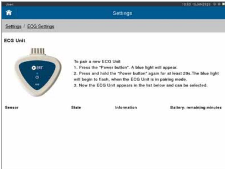
1. On your ECG Unit press and hold the power button until the blue LED blinks fast. This will take approximately 20 seconds.
