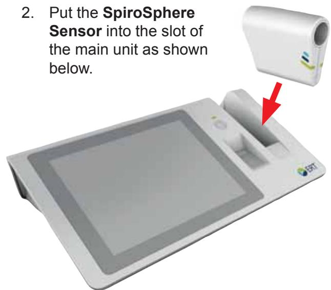
3. Use the Power On switch located at the front of the main unit to switch on the **SpiroSphere Main Unit**.
