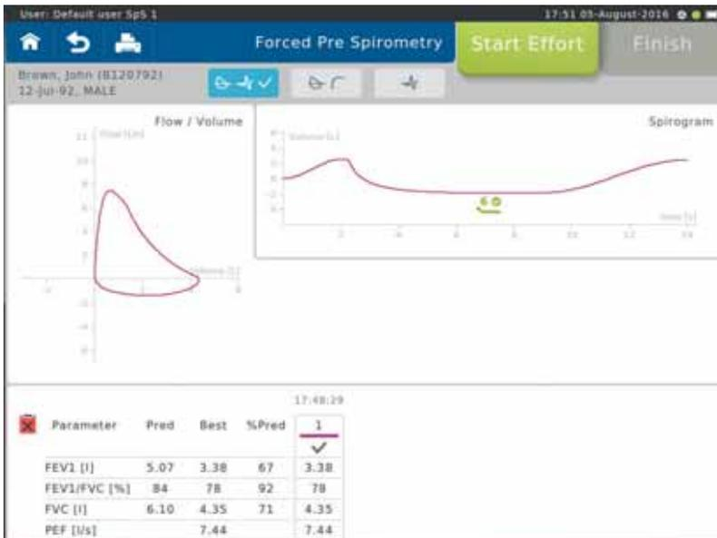
The upper left part of the chart section shows the recording of the flow-volume loop. The upper right part shows the volume-time tracing.
