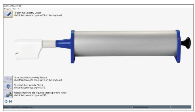
2. Use the 3-L calibration syringe for calibration. Connect the calibration syringe to the wireless spirometry sensor unit.
