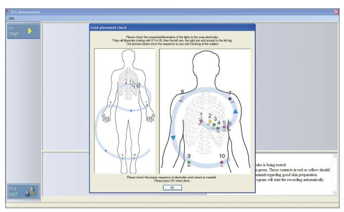
To enable an easy check of the electrode placement, the system will illuminate the electrodes in a fixed sequence.
