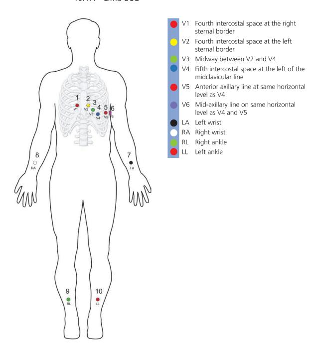
When connecting the electrodes to MasterScope ECG, the tiny and fast potential differences originating from the heart can be detected on the surface of the body between either two individual electrodes or between one individual electrode and a group of combined electrodes and recorded by MasterScope ECG.
