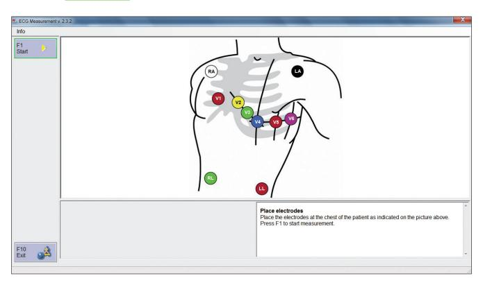
The electrode test program automatically checks whether the electrodes are in good contact with the skin. If a contact is poor, the respective electrode will immediately be indicated on the screen and directly at the electrode.
