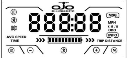
Mode Pressing the "M" (Mode) symbol allows the user to change between current speed, average speed, trip time, trip distance, odometer, and speaker volume.
