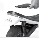
6. Install seat cover plate (included in carton) using the four Allen screws removed in step number two above.
