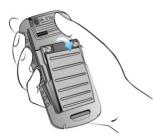
3. Insert the battery and push it into the battery slot such that the three metallic contacts at the bottom of the battery are aligned with the metallic contacts within the battery compartment.
