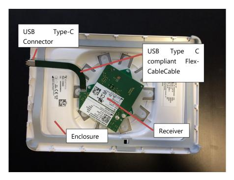
The following pictures shows the enclosure for both Wireless Receiver and tablet with Receiver and tablet mounted. The tablet is connected with the Receiver using an USB-cable (see picture above and section "Integration into products".
