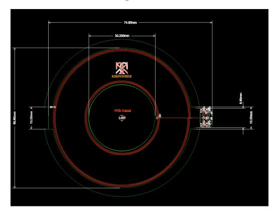
As shown in various EMC tests, no intended radiation is used to transmit data. All information is transmitted using the principle of near field coupled coils utilizing a carrier frequency of 2MHz. The coil area used is 440 mm<sup>2</sup>.
