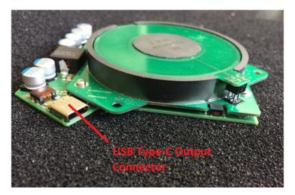
The Wireless Power Receiver shall be mounted using the mounting holes provided by the manufacturer. M3 screws are suitable, e.g. Screwerk STP 3803000803 or comparable. The cable to supply the load shall be USB Type-C compliant.
