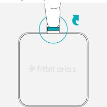
2. Remove the batteries.
