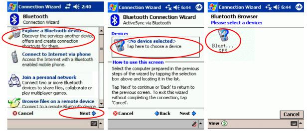
Mini Solar Bluetooth GPS Receiver User Manual 6) Back to the [Explore a Bluetooth device] as below. Click [Next] to list service on Bluetooth GPS. [SPP slave] should appear in the service list box, click it and click [Next] to finish shortcut creation. Don't forget to uncheck the secure connection box.
