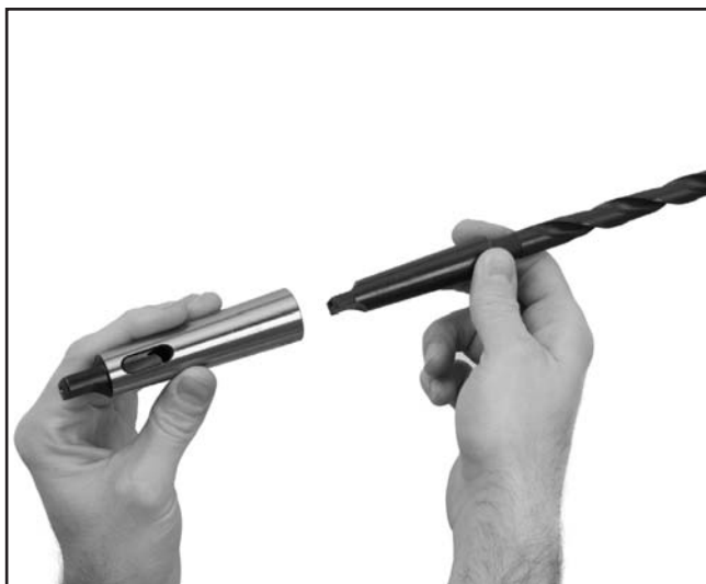
Figure 13. Installing tapered tooling into a drill sleeve.
