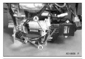
• Connect the handtester to the adapter and Engine ground (or Battery Terminal (-)).
