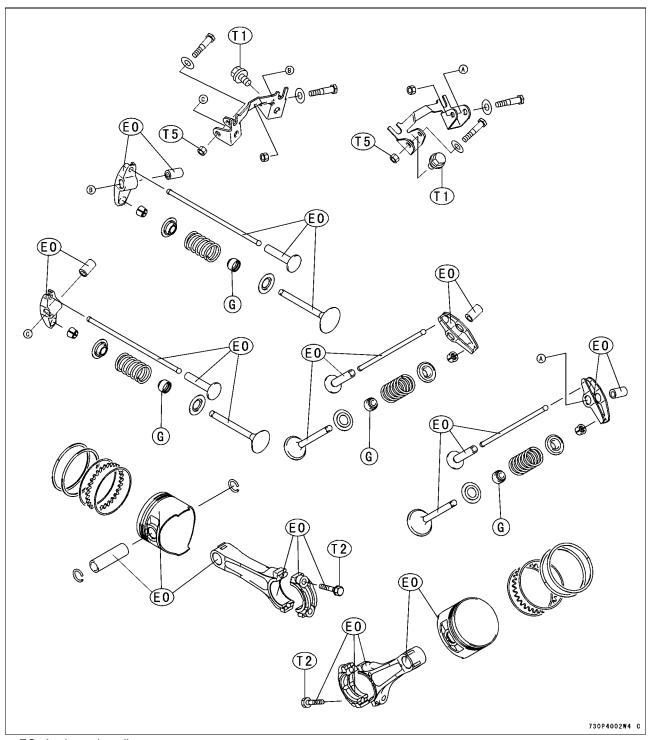
EO: Apply engine oil. G: Apply grease.
