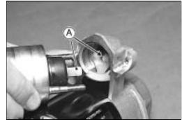
• Fit the notch [A] in the (-) lead grommet onto the projection [B] on the
