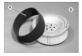
• Clean the paper element [B] by tapping it gently on a flat surface to remove dust. If the element is very dirty, replace it with a new one.
