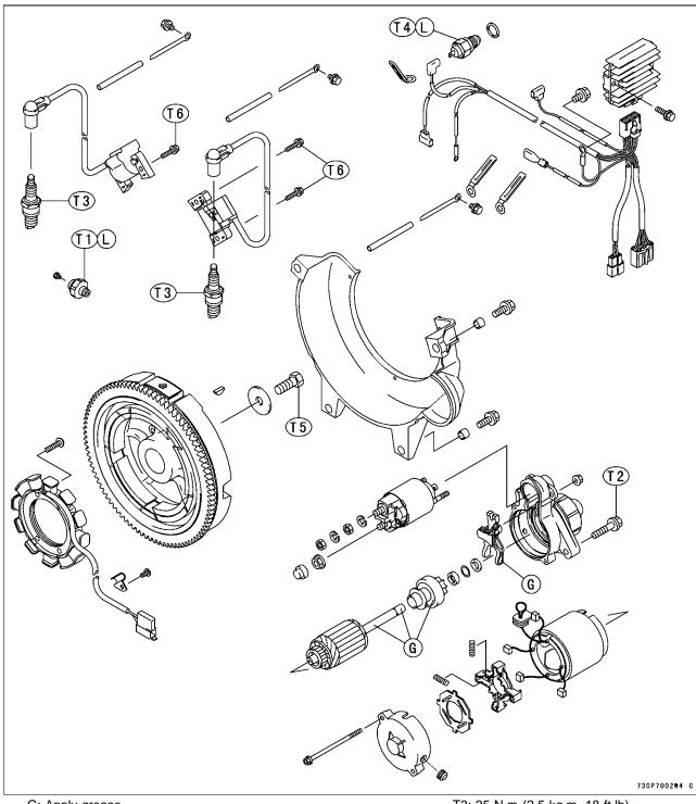
G: Apply grease. L: Apply a non-permanent locking agent. T1: 15 N·m (1.5 kg·m, 11 ft·lb) T2: 20 N·m (2.0 kg·m, 15 ft·lb) T3: 25 N·m (2.5 kg·m, 18 ft·lb) T4: 27 N·m (2.8 kg·m, 20 ft·lb) T5: 56 N·m (5.7 kg·m, 41 ft·lb) T6: 3.4 N·m (0.35 kg·m, 30 in·lb)
