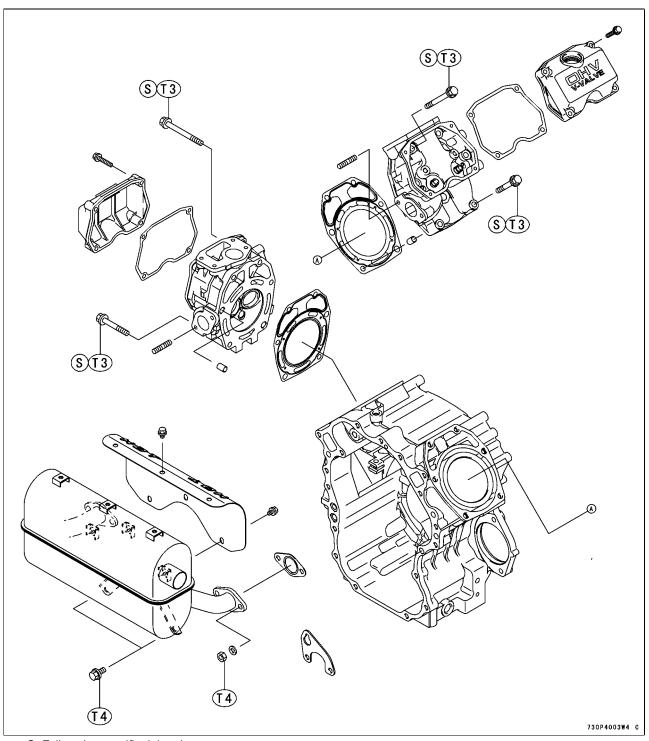
S: Follow the specific tightening sequence. T3: 27 N·m (2.8 kg·m, 20 ft·lb) T4: 20 N·m (2.0 kg·m, 15 ft·lb)
