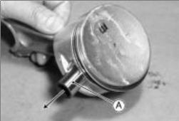
• Remove the top and second rings with piston ring pliers.
