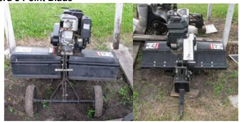
Pull Behind External Engine Tiller (does not run off the lawn tractor, the tractor only pulls it as it the tiller has an independent power source)
