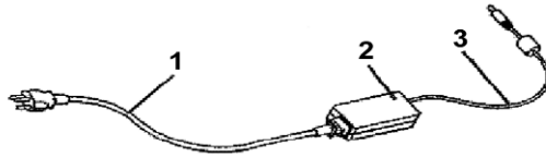
1. AC Power Cord / 2. AC Adapter / 3. DC (Direct Current) Cord
