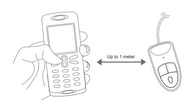
Prior to using your Bluetooth Clip Headset for the first time, you must pair it with a Bluetooth-enabled mobile handset. Your headset can be paired with up to 8 mobile handsets at a time by following the simple steps in the next page.
