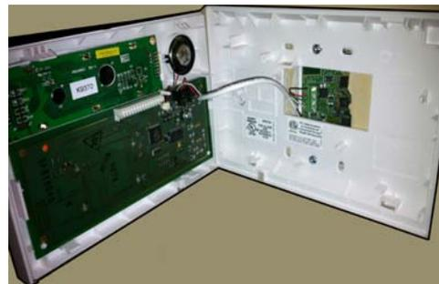
**J.** Return AC power and then the red and black flying lead from the battery located in the Vista 20P alarm panel.
