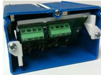
**G.** If the existing Vista 20P keypad was not mounted on an approved recessed electrical enclosure box, then use the included Panel Interface plastic holder as a guide to cut a recess opening to mount the device.
