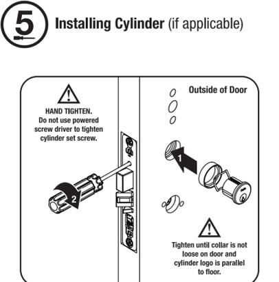
**STOP** Test cylinder operation before continuing.
