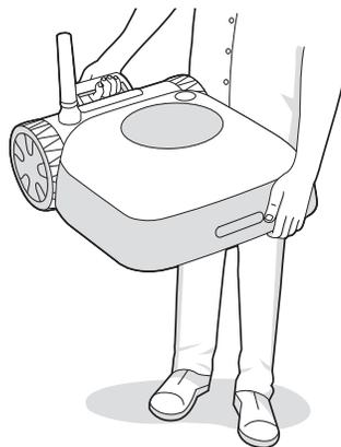
**Warning:** Always press the STOP button before lifting or carrying the robot.
