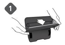
Set Mint Plus on its end and remove the cleaning pad.
