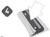
Caution: Make sure the cleaning cloth does not drape into the middle channel between the gripping strips as this could impede sensor functions and safe operation.
