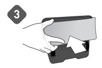
Re-attach the cleaning pad. Magnets will help it snap back into place.
