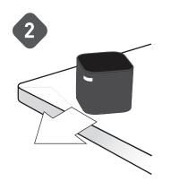
Place the NorthStar Navigation Cube on a table or counter top, pointing the blue light away from walls and toward the middle of the room.
