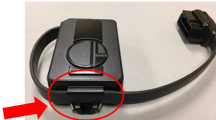
Coil the cable, securing it to the enclosure
