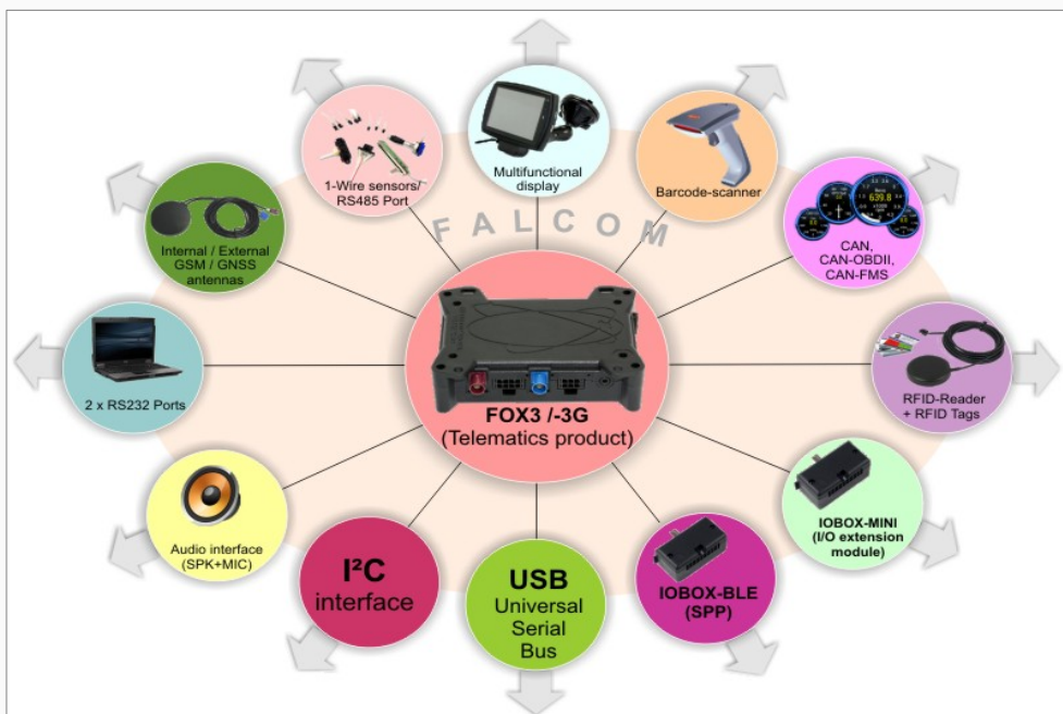
Figure 1: FOX3-2G/3G/4G networking and interfaces to peripheral devices.
