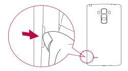
2 Slide the SIM card into the lower slot for the SIM card as shown in the figure on the next page. Make sure the gold contact area on the card is facing downward.
