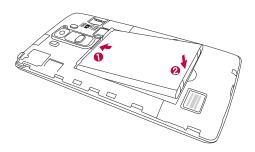
4 To replace the cover onto the device, align the back cover 1 and press it down until it clicks into place 2.
